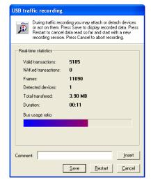
Note that the USB Tracker's real-time recording and analysis capability relies on a USB 2.0 connection. As such, the vendor notes that two host controllers comprise an optimum set-up. The first controller is used to connect the peripheral to be tested, and the other controller is used to record your data.
