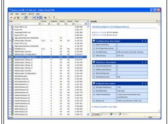
A second window gives more details. To make it easier to identify packets, the system's software includes filtering and packet-coloring functions. It also lets you select levels of detail. Also, the information derived from bus traffic is equated with references to the USB standard.
