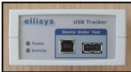
**Photo 2**—You don't need anything but this little box, a downloadable software application, and three USB cables to help unlock the mysteries of USB. It costs less than \$1000.
