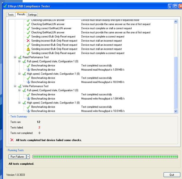
The Ellisys Device Compliance Testing software, included with the USB Explorer 260 Generator, automatically verifies the compliance of devices against the USB specification and classes specifications such as HID and Mass Storage.
