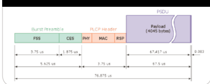
Figure 5 – Burst Frame Elements Duration at 480 Mbps 4
